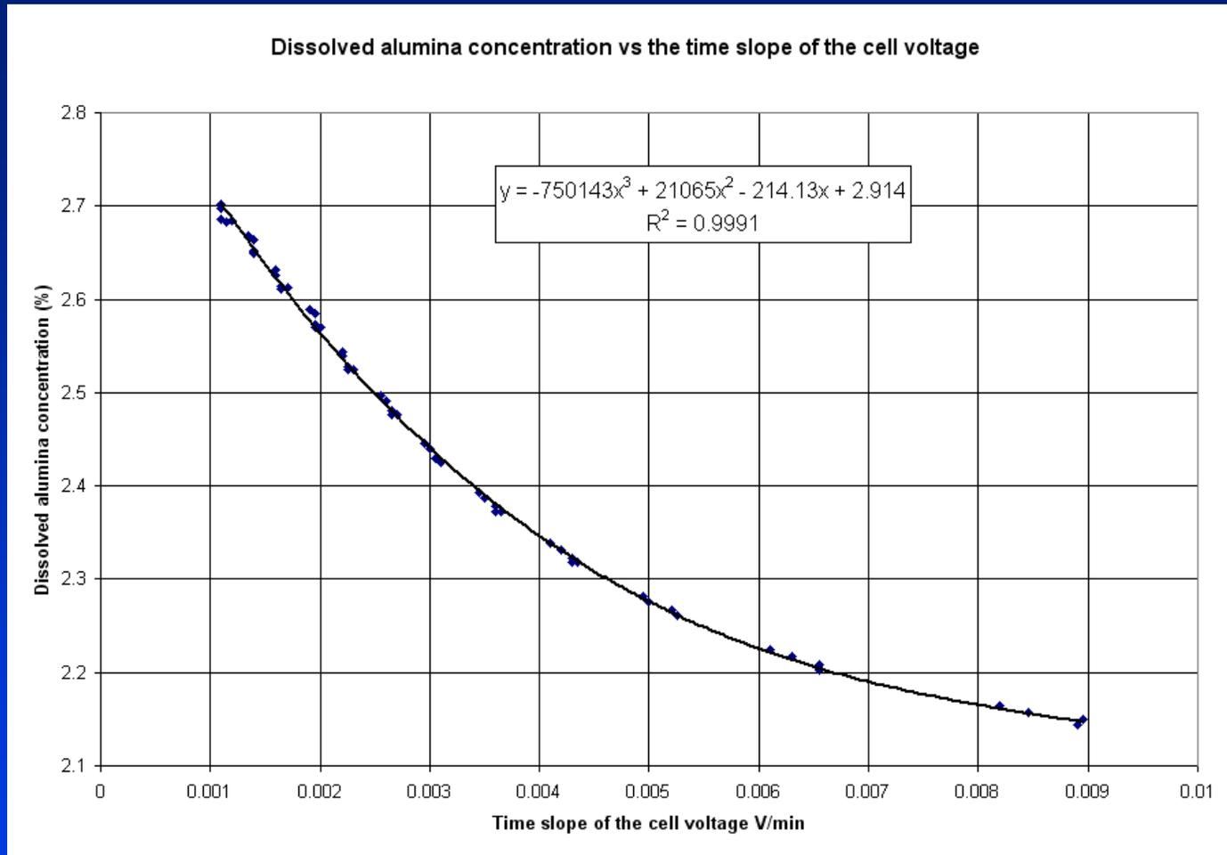
Tests performed on Dyna/Marc cell simulator indicates that this correlation does exist even if it is not linear on a very wide range of alumina concentration variation and depends on a lot on factors influencing the cell resistance and the dynamics of the alumina dissolution.
