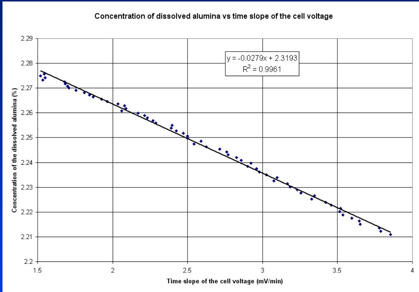
For a more restricted range of alumina concentration variation which corresponds to the typical range the *In Situ* controller would be able to operate the cell and for a different value of the alumina dissolution constant, a linear correlation was obtained.
