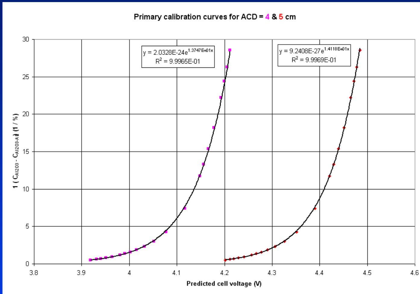
In is quite easy to generate this correlation for any combination of cell conditions using published cell voltage break down equations like those published in [Introduction to Aluminium Electrolysis: Understanding the Hall-Heroult Process](#), that happen to be the ones used by Dyna/Marc.
