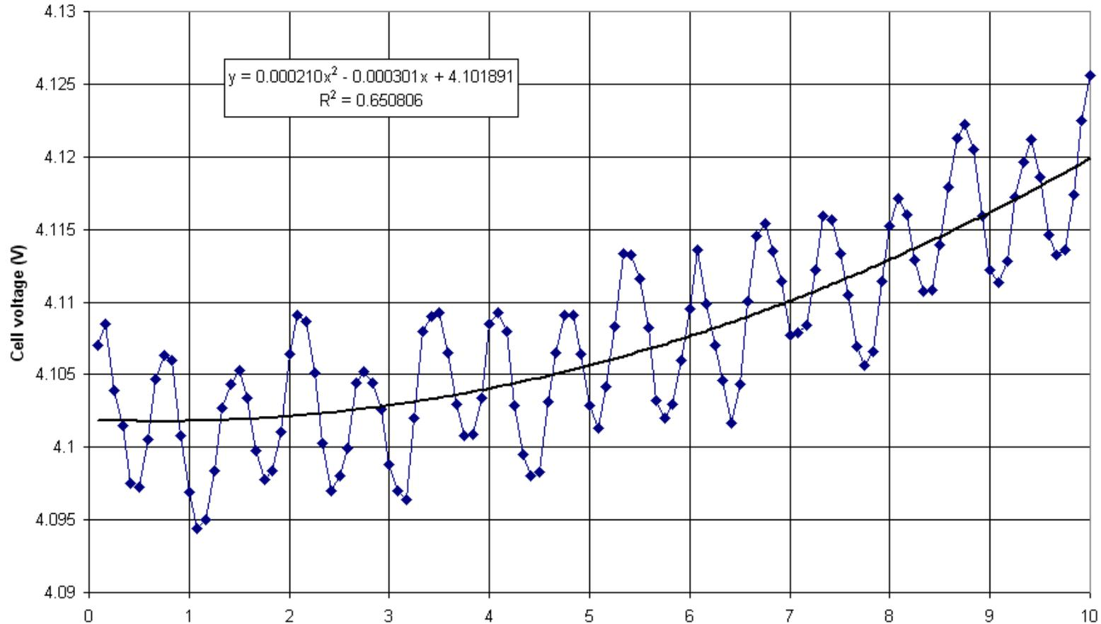
Prediction of the current noise free slope of the normalized cell voltage:  $2 \cdot 0.00021 \cdot 10 - 0.000301 = 0.0039 \text{ V/min}$
