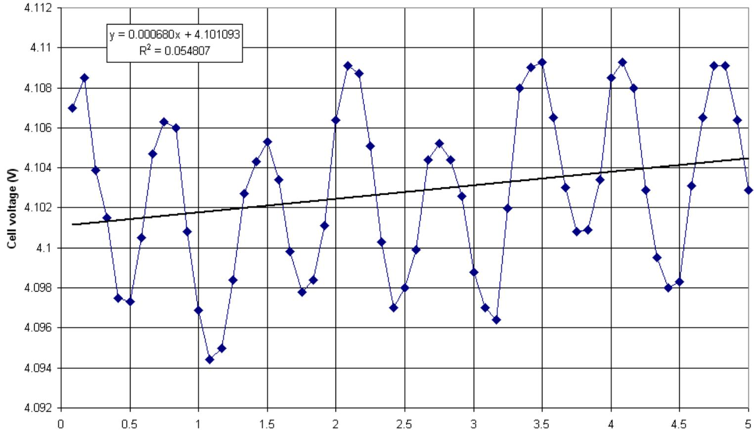
Prediction of the current noise free slope of the normalized cell voltage: 0.00068 V/min
