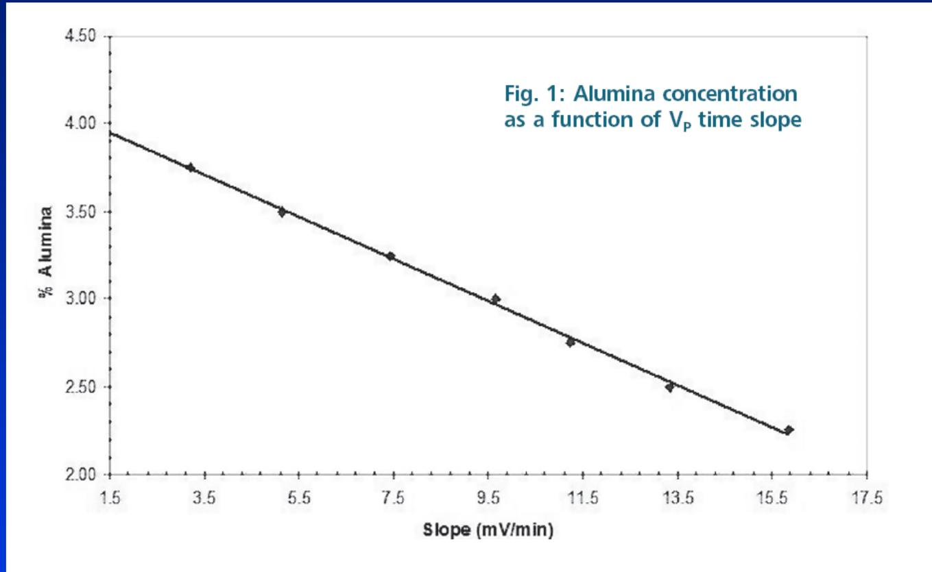
The key concept of the *In Situ* control logic algorithm is the assumption that there is a correlation between the estimated slope of the noise free normalized cell voltage (called time slope of  $V_p$  in previous *In Situ* papers) and the alumina concentration during a no feed observation period.
